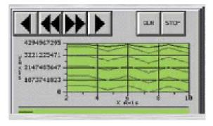
Track up to 6 variables in one trend graph. Acquire and store data. Perform stasistical proces control. Scripting allows logical and mathematical operations on PLC data
